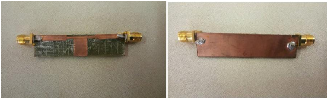
Figure 7. Fabricated Open-Circuited Stub 2GHz Low Pass Filter
